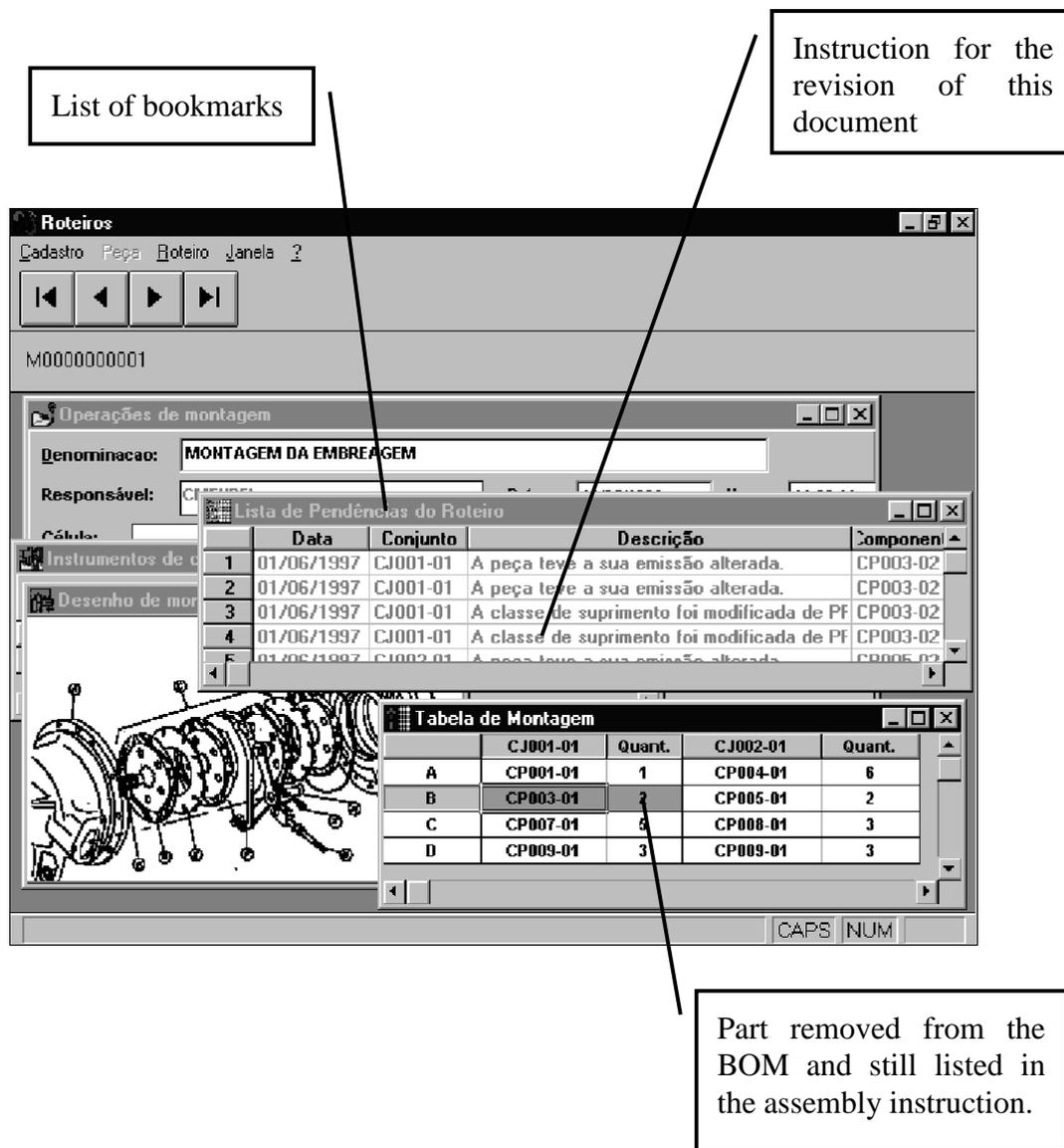
Figure 3: Control of inconsistencies in an assembly instruction
